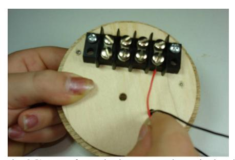
Attach the RED wire from the buzzer to the right hand screw on the terminal block.
