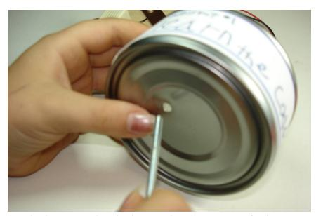
Insert the bolt into the hole in the bottom of the can.
