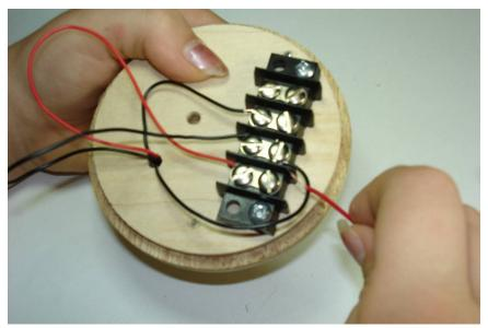
Now attach the RED wire from the battery clip to the terminal block screw directly opposite the RED buzzer wire.
