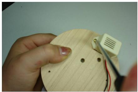
Mount the buzzer using the 2 tiny screws.
