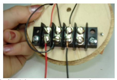
And the BLACK battery clip wire attaches 2 screws over and directly opposite the second metal strip wire.
