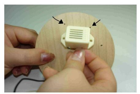
Locate the 2 holes for the buzzer on the top side of the board.
