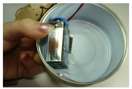
Place the battery inside the can and in the smaller area to one side of the bolt.
