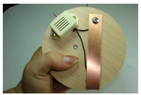
Now thread these 2 wires down through the hole next to the buzzer. Make sure that the lower wire runs by the second hole.
