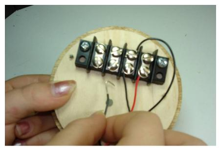
Now attach the other wire from a screw on the top side metal strip to the terminal block screw right next to the BLACK buzzer wire. Again, it is better to make a little 'hook' in the wire to hold it around the screw when you tighten it down.
