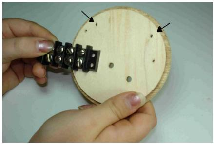
Locate the 2 holes for the terminal block on the bottom side.
