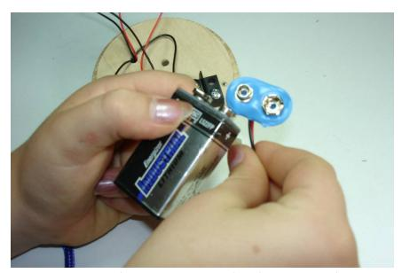
Insert a battery into the battery clip.
