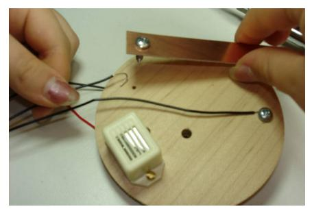
Put a screw through the hole on the metal strip and then screw it down onto the board with the wire hooked around the screw underneath the strip.
