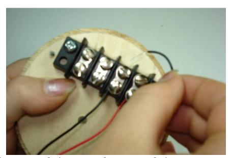
Now loop one of the wires from one of the screws on either end of the metal strip on the top side and attach it to the terminal block using the screw directly opposite the BLACK buzzer wire.
