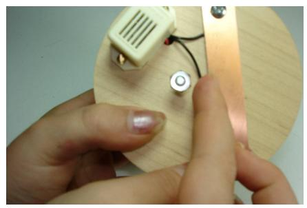
Now place the cover on the can, with the bolt coming out of the other large hole, and carefully stuff all the loose wires down inside the can.
