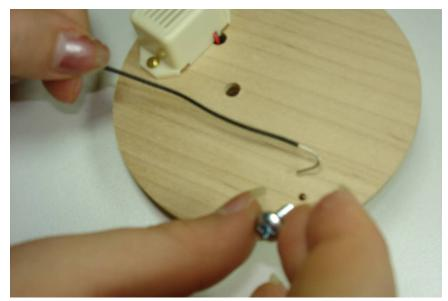
Put a 'hook' in one of the pieces of wire. Screw it down onto the board using one of the larger screws.
