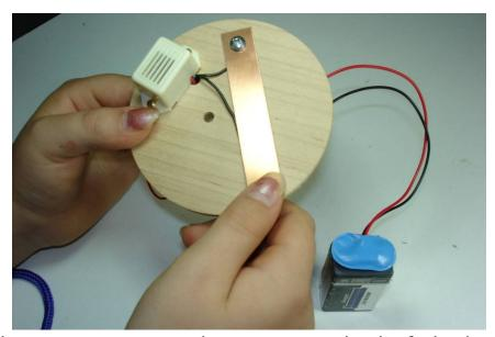
And now you can test the circuit to check if the buzzer sounds when you press down on the metal strip. If the buzzer is ALWAYS sounding, bend the metal strip up a little until it doesn't touch the screw underneath it. Then press the metal strip down and test the 'key' action.
