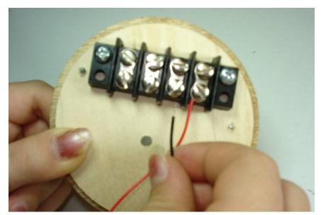
Attach the BLACK buzzer wire to the terminal screw right next to the red buzzer wire.
