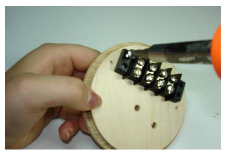
Screw the terminal block onto the board using 2 large screws.
